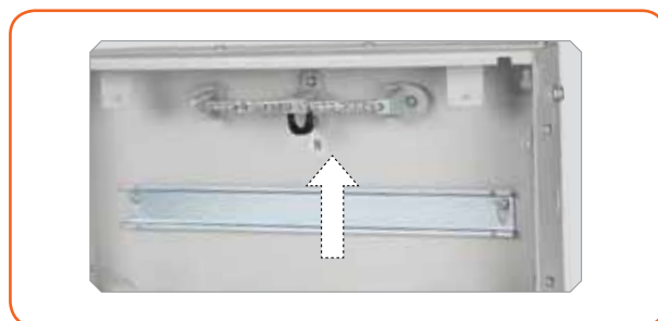
Remove link to use split neutral provision • Use 1st neutral link for mains supply • Use 2nd neutral link for stand by supply
