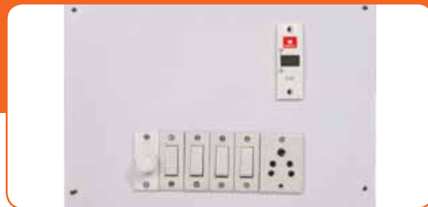
Screw mount its front plate on the switchboard.
